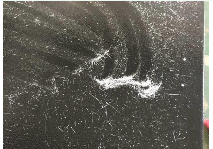
66 remark-poly foam dust stuck on the cabinet surface (3)
