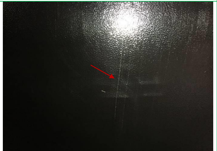
68 defect-scratch mark on the surface-mi (1)
