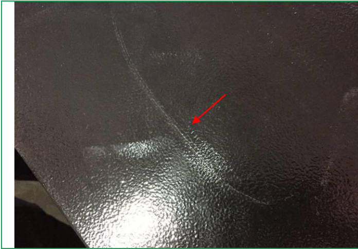
69 defect-scratch mark on the surface-mi (2)
