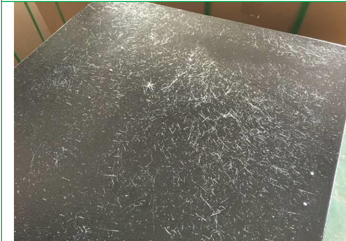
65 remark-poly foam dust stuck on the cabinet surface (2)
