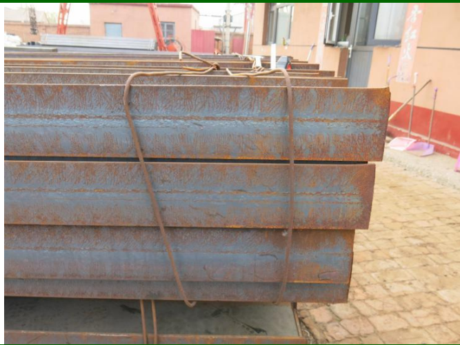
49. Defect: 100% sample size found the rust mark on surface
