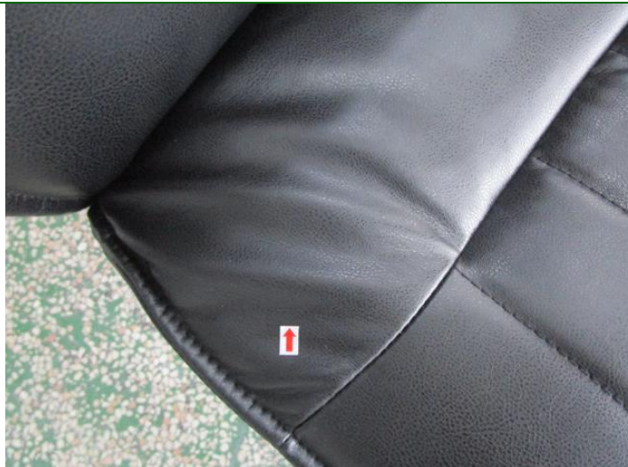
311. Defect-25089789 Wrinkle surface - major
