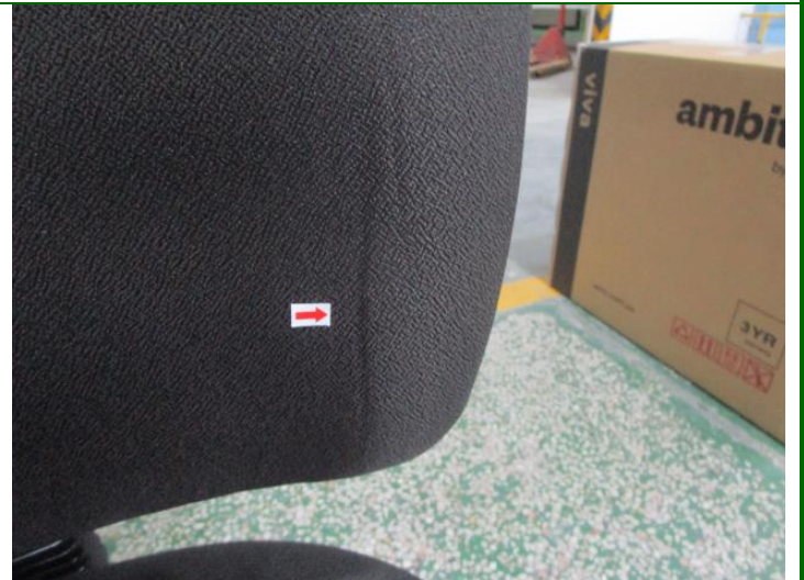
312. Defect- 25089763 Wrinkle surface - major
