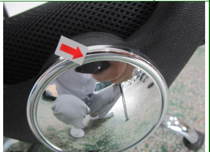
314. Defect- 18902570 - Scratch mark - minor
