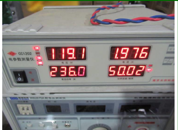
164. Power Consumption Check
