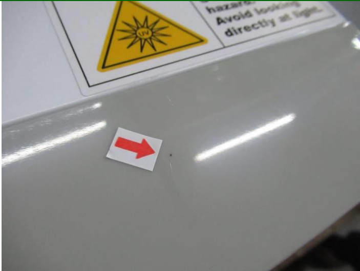
197. Defect- Black mark on surface-Minor
