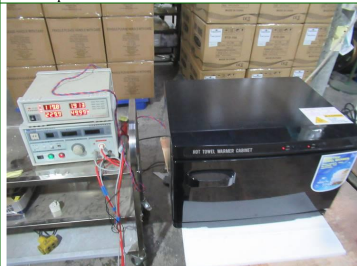
161. Power Consumption Check
