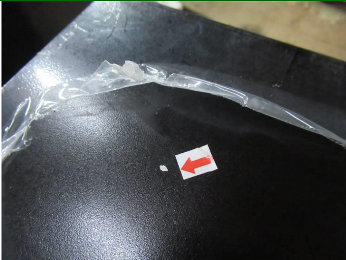
195. Defect- Painting peel off- Minor
