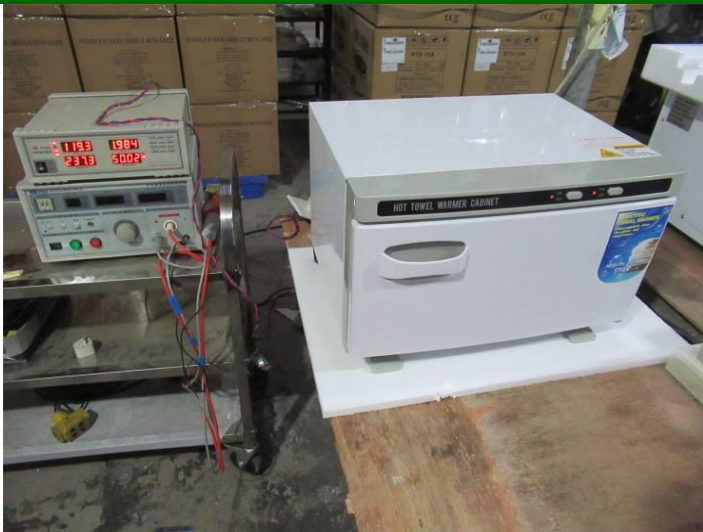
163. Power Consumption Check
